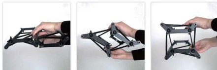
Unfolding of Truss module
